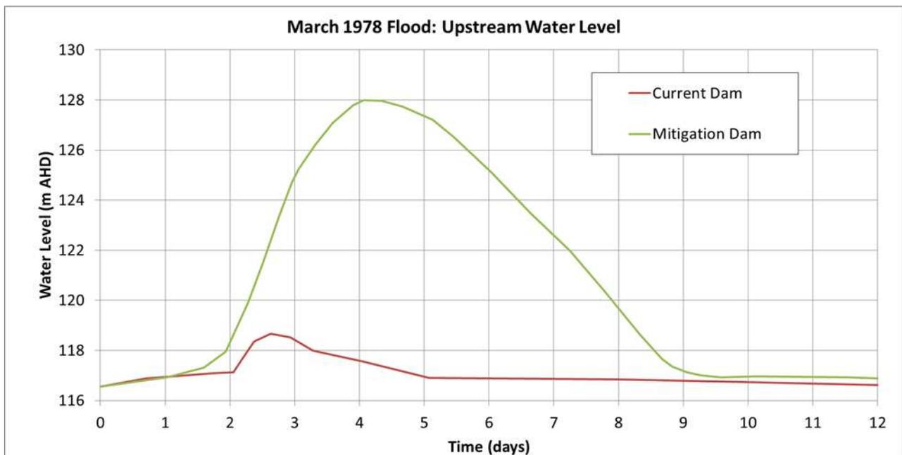
Figure 3 March 1978 Flood, Upstream Water Levels
