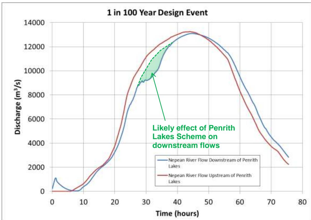
Figure 1 Likely Effect of the Penrith Lakes Scheme on Downstream Flow
